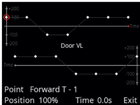
In Manual Setup you can set seven travel points in time and position for each function; forward and reverse processes are individually variable.
