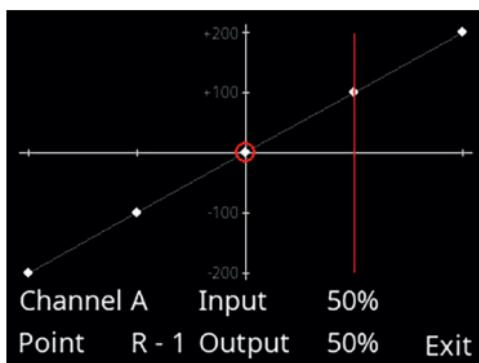
The procedure is very simple: use buttons I and II to select the point on the curve which you wish to change, then press the SET button. The servo automatically moves slowly to the corresponding point. Now you can adjust the servo curve at this point using buttons I and II.
